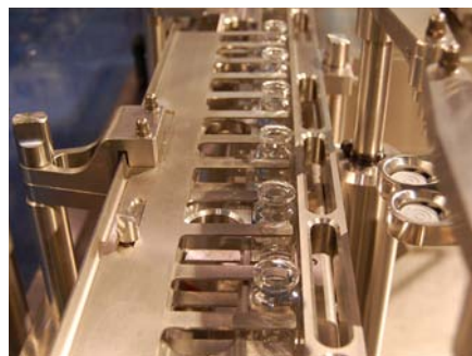
Easy changeover between vial sizes in few minutes, gentle transport of vials and no contact with machine parts during check weighing. Simply by using a walking beam.
